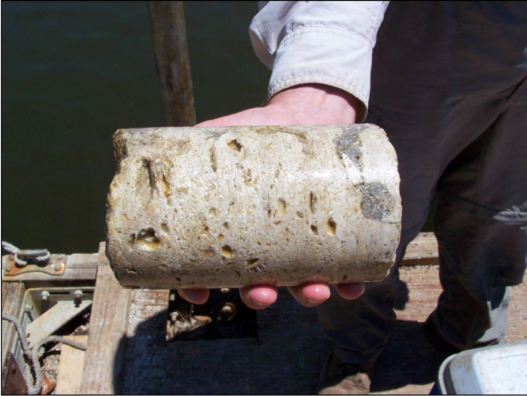
Rock core recovery from rock boring depth of 0ft to 1ft
