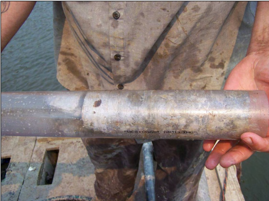
Rock core recovery from rock boring depth of 6ft to 8ft
